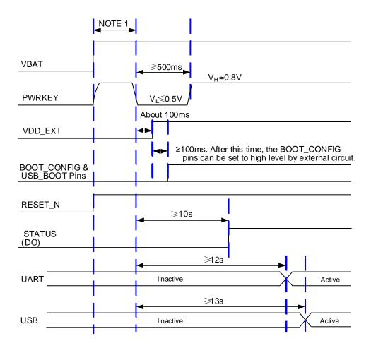
Figure 12: Timing of Turning on Module
