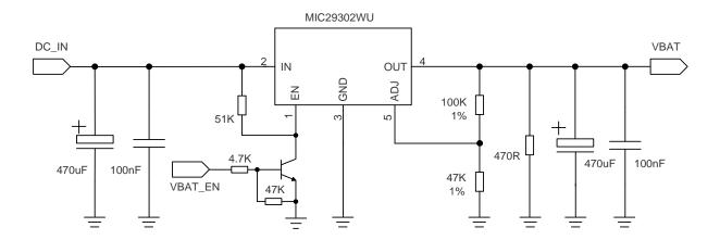
Figure 9: Reference Circuit of Power Supply
