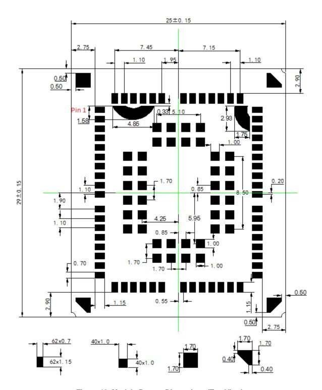
Figure 42: Module Bottom Dimensions (Top View)
