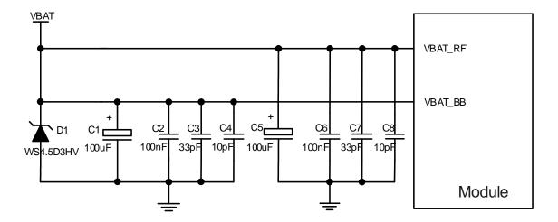
Figure 8: Star Structure of Power Supply
