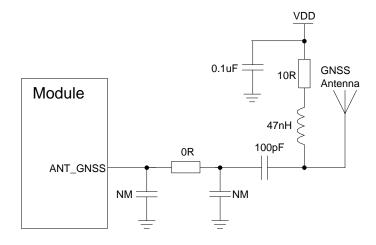
Figure 35: Reference Circuit of GNSS Antenna
