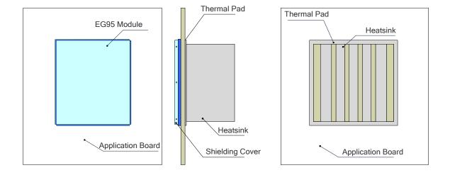
Figure 40: Referenced Heatsink Design (Heatsink at the Backside of Customers' PCB)
