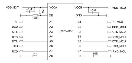
Figure 20: Reference Circuit with Translator Chip
