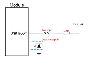
Figure 28: Reference Circuit of USB\_BOOT Interface
