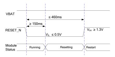
Figure 16: Timing of Resetting Module
