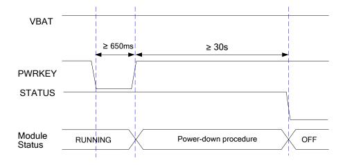
Figure 13: Timing of Turning off Module
