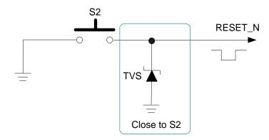
Figure 15: Reference Circuit of RESET\_N by Using Button
