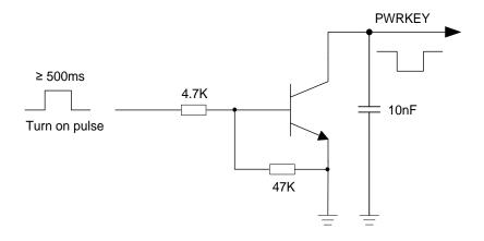
Figure 10: Turn on the Module Using Driving Circuit
