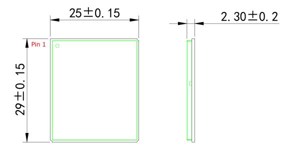
Figure 41: Module Top and Side Dimensions
