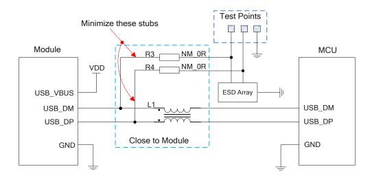
Figure 19: Reference Circuit of USB Interface
