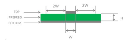
Figure 31: Microstrip Line Design on a 2-layer PCB
