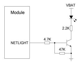
Figure 26: Reference Circuit of Network Status Indicator
