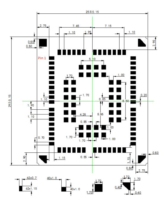
Figure 43: Recommended Footprint (Top View)
