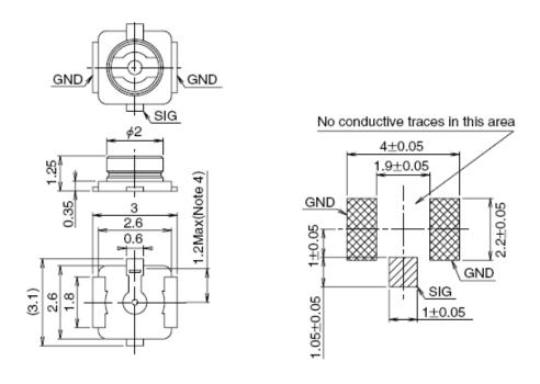
Figure 36: Dimensions of the U.FL-R-SMT Connector (Unit: mm)
