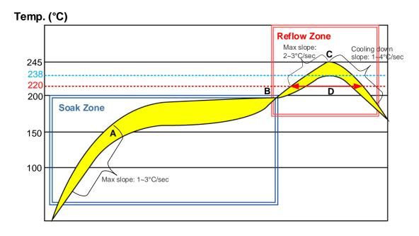
Figure 46: Reflow Soldering Thermal Profile
