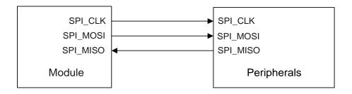
Figure 25: Reference Circuit of SPI Interface with Peripherals
