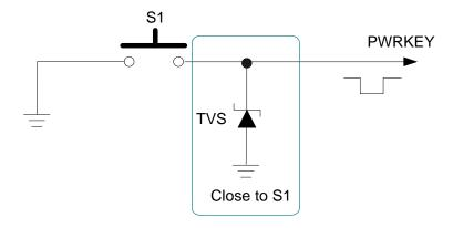
Figure 11: Turn on the Module Using Button
