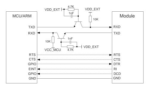
Figure 21: Reference Circuit with Transistor Circuit
