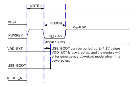
Figure 29: Timing Sequence for Entering Emergency Download Mode
