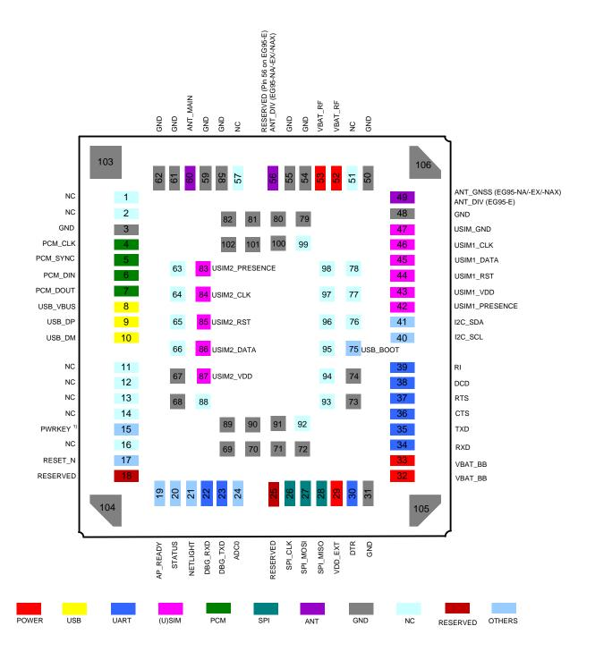
Figure 2: Pin Assignment (Top View)
