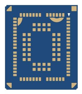
Figure 45: Bottom View of the Module
