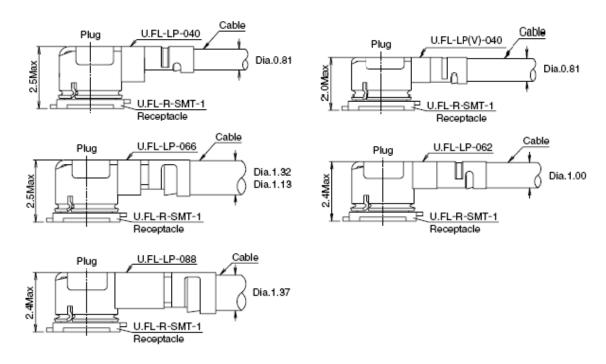
Figure 38: Space Factor of Mated Connector (Unit: mm)
