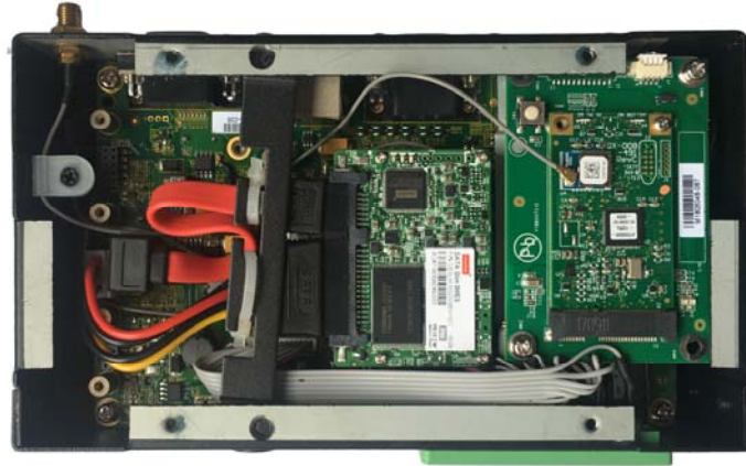
Bottom View for embedded modules (1xHalf PCIe slot under the 1xPCIe slot)
