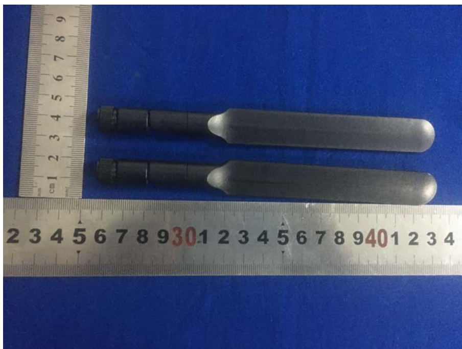
4G Antenna View
