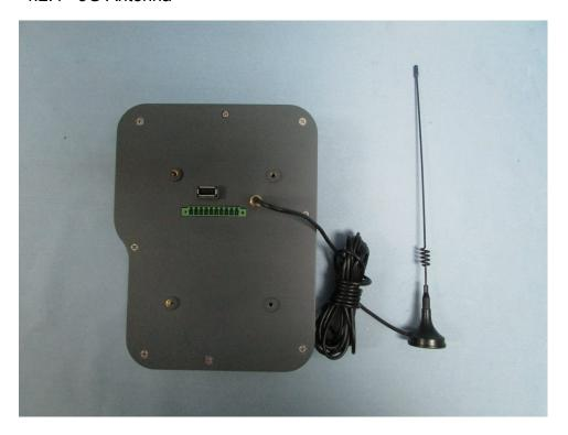
The antenna is only being used to the EUT. The antenna gain is 5.12 dBi for Cellular & 6.12 dBi for PCS
