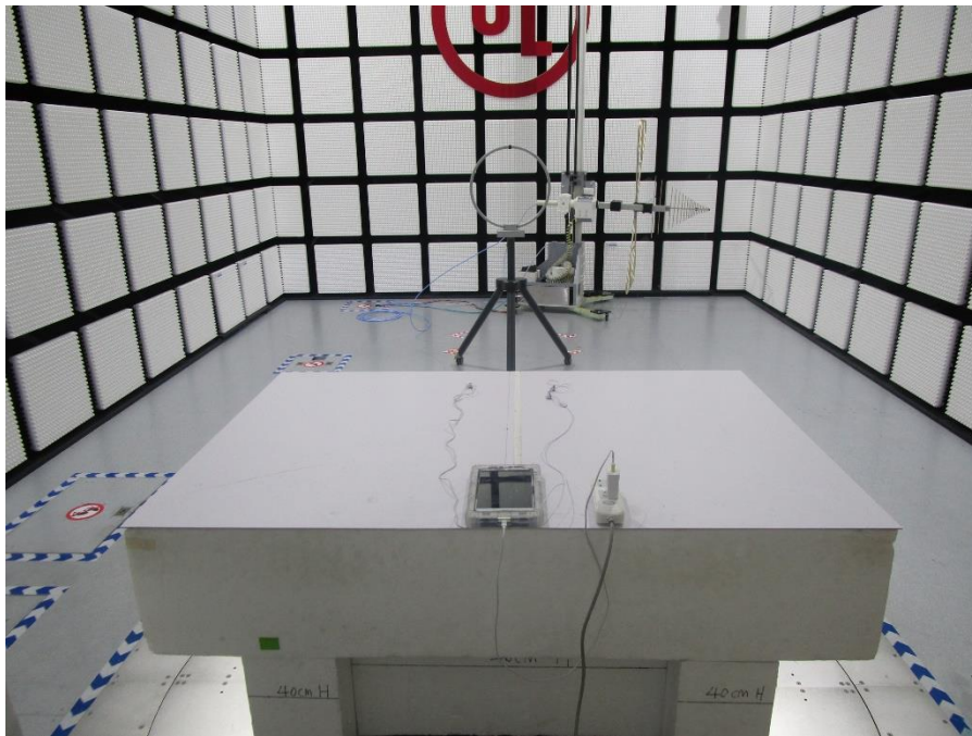
RADIATED RF MEASUREMENT SETUP (Below 30MHz)
