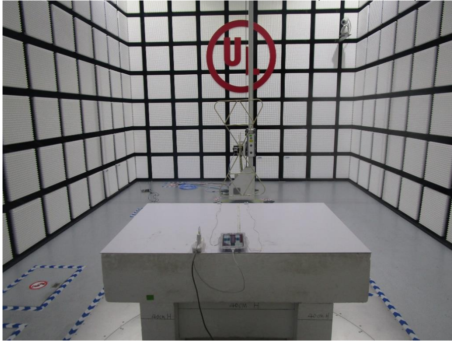
RADIATED RF MEASUREMENT SETUP (Below 30MHz)
