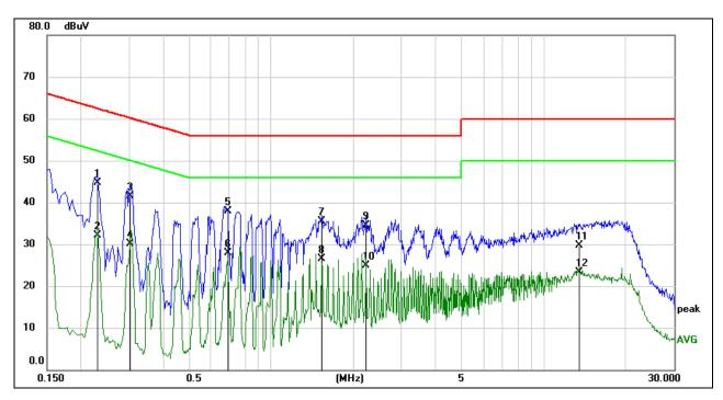
LINE L RESULTS with modified sample (transmitter terminated into a dummy load)
