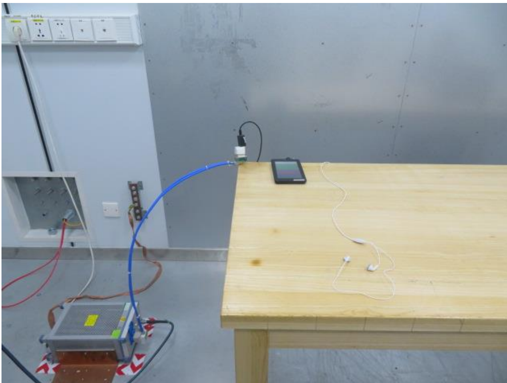
POWERLINE CONDUCTED EMISSIONS MEASUREMENT SETUP
