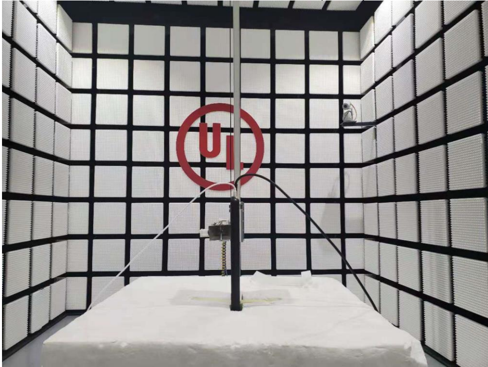
RADIATED RF MEASUREMENT SETUP (30MHz~1GHz)
