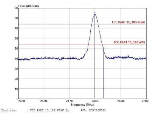
Preamp Cable Factor Loss Antenna Level Limit Margin Remark Item Freq Read Level Factor dBuV MHz dBuV dB dB dB dBuV dBuV 1 2480.00 86.91 27.59 34.97 4.00 83.53 74.00 9.53 Peak 27.59 2 2483.50 51.48 34.97 4.00 48.10 74.00 -25.90 Peak
