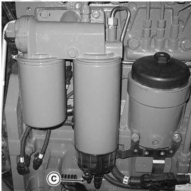
Water Separator Drain Valve—9.0 L Shown
