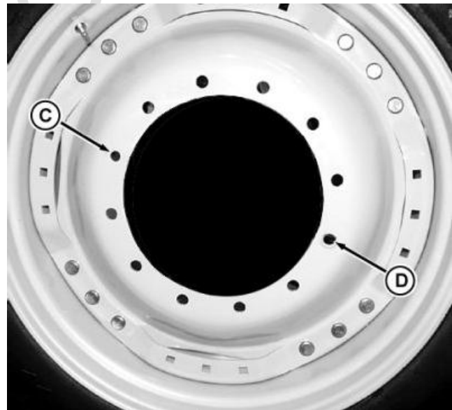
A—Wheel-to-Rim Tight Fit Hole C—Disk-to-Hub Tight Fit Hole B—Wheel-to-Rim Slot Fit Hole D—Disk-to-Hub Slot Fit Hole
