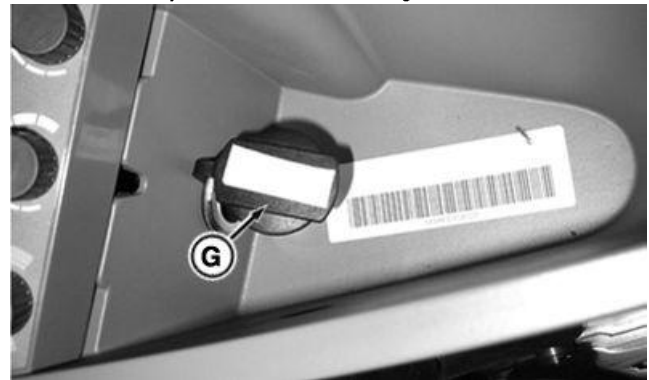
Accessory Electrical Outlet In Storage Box
