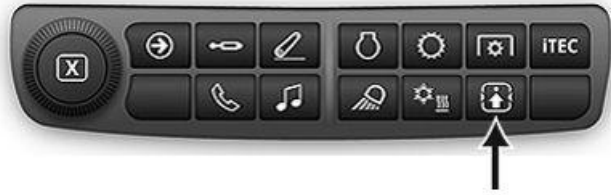
Generation 4 Controls Setup Shortcut Button
