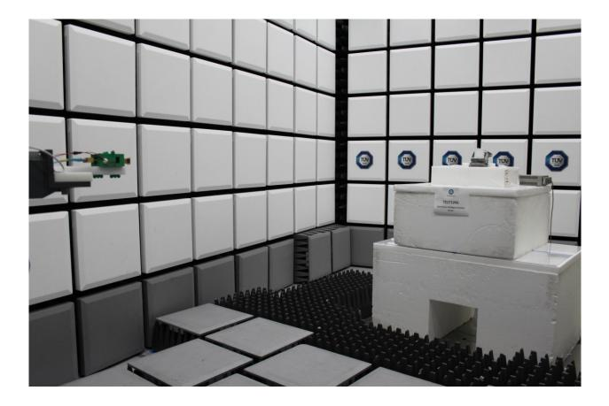
Radiated Emissions Test Setup (above 40GHz)
