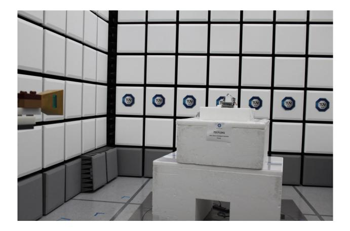
Radiated Emissions Test Setup (18GHz to 26GHz)
