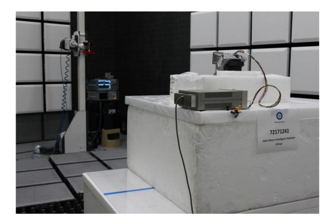
Radiated Emissions Test Setup (1GHz to 18GHz)
