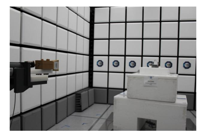
Radiated Emissions Test Setup (26GHz to 40GHz)
