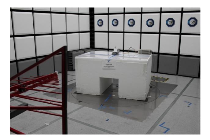
Radiated Emissions Test Setup (30MHz to 1GHz)
