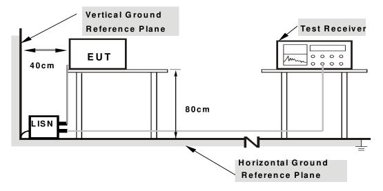
Note: 1.Support units were connected to second LISN. 2.Both of LISNs (AMN) are 80 cm from EUT and at least 80 from other units and other metal planes
