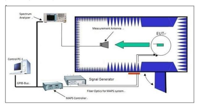
Figure 1. 2D antenna pattern test system.
