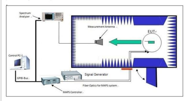
Figure 1. 2D antenna pattern test system.
