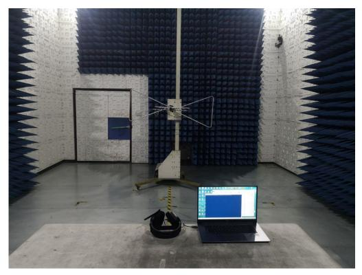
RADIATED EMISSION TEST SETUP ABOVE 1GHZ
