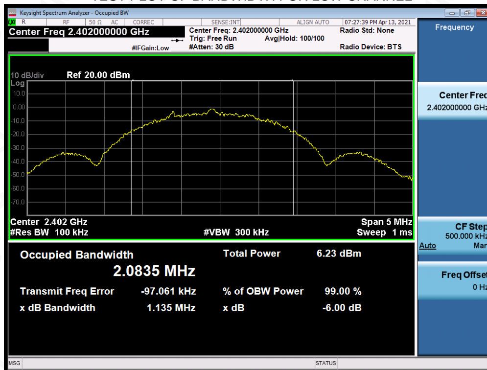
TEST PLOT OF BANDWIDTH FOR LOW CHANNEL
