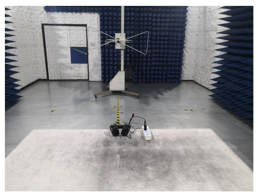
RADIATED EMISSION TEST SETUP ABOVE 1GHz
