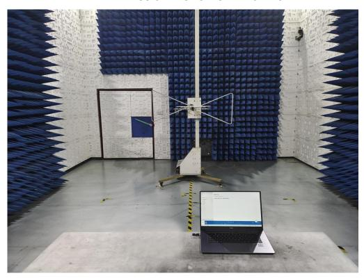
RADIATED EMISSION TEST SETUP ABOVE 1GHZ
