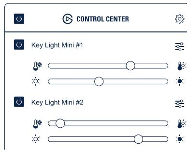
Use Control Center to switch Key Light Mini on/off, adjust brightness, fine-tune color temperature and configure advanced settings.
