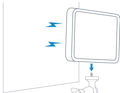
Place Key Light Mini on a flat surface, attach it to a 1/4" mount (e. g. Elgato Multi Mount) or stick it onto a magnetic surface.
