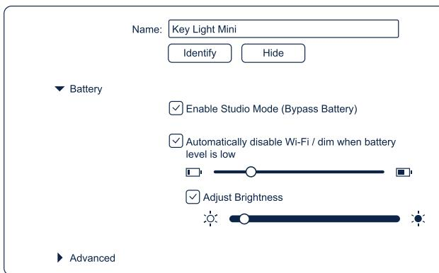
If your Key Light Mini is connected to mains all the time, enable Studio Mode to completely bypass the battery. This mode will help to extend the lifetime of your battery and avoid overheating during long hours of operation. Enable Energy Saving Mode to turn off Wi-Fi and dim the light if the battery level is low. Set your personal threshold for activating Energy Saving Mode by adjusting the battery level.
