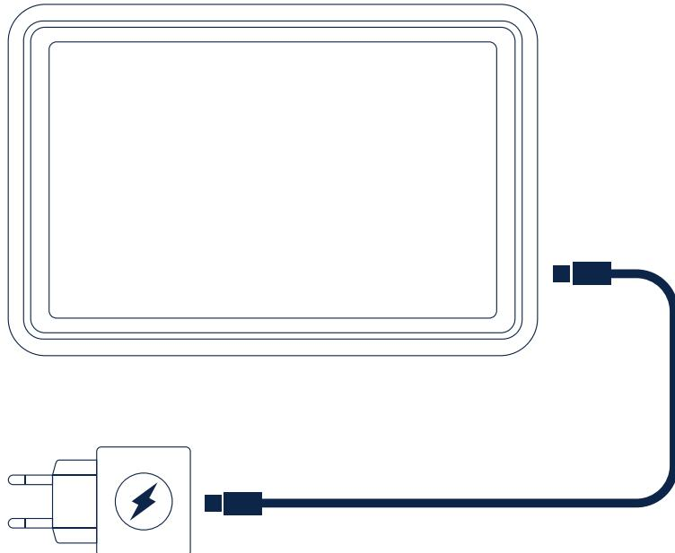
Connect Key Light Mini with the supplied USB cable to a 5 V USB charger with min 2.4 A. The charging process will start automatically and the charging level will be shown by the battery status indicator. Once charging is complete (after around 60-100 min) all LEDs will be steadily lit.
