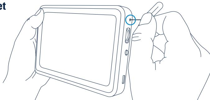
Power on Key Light Mini. Push and hold the Reset button with a small tool for at least 10 seconds until the light flashes 3 times. Then release the button. Key Light Mini will restart automatically after a few seconds.
