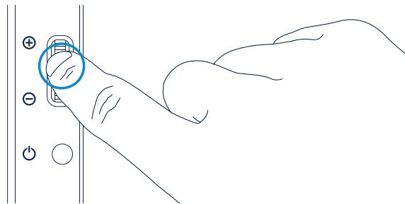
Key Light Mini is in brightness mode by default. Briefly press the jog wheel to enter color temperature mode (Key Light Mini will flash twice), and repeat to return to brightness mode (Key Light Mini will flash once). Push the jog wheel up/down to adjust the intensity of brightness or color temperature.
