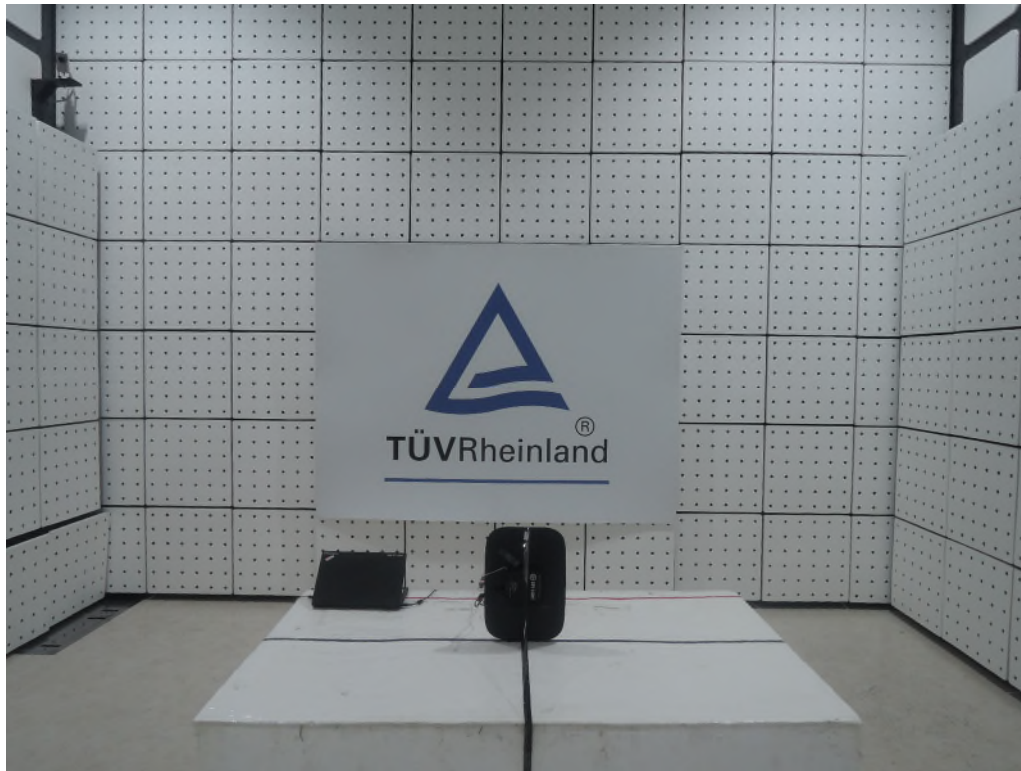
Photograph 2: Set-up for Spurious Emissions (Back View 1)
