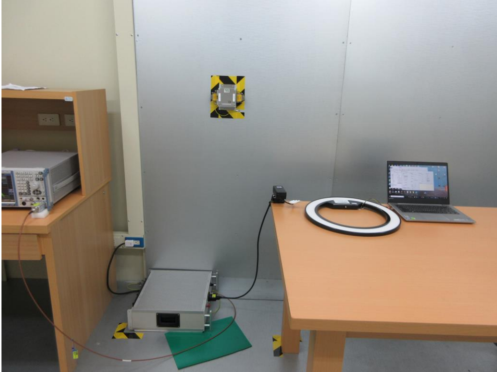
Photograph 7: Set-up for AC Mains (Front View)
