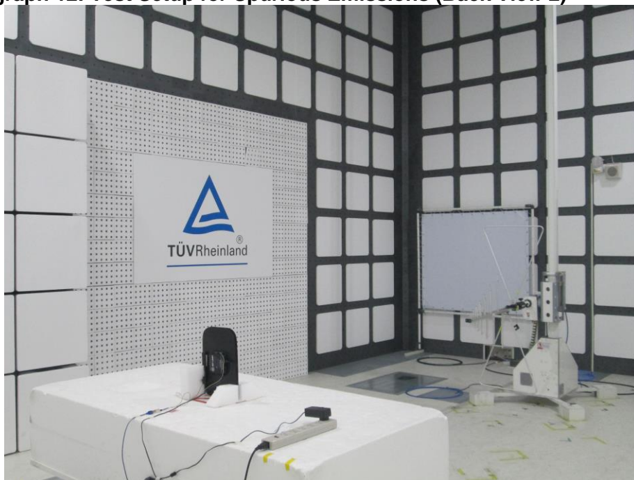
Photograph 12: Test Setup for Spurious Emissions (Back View 2)
