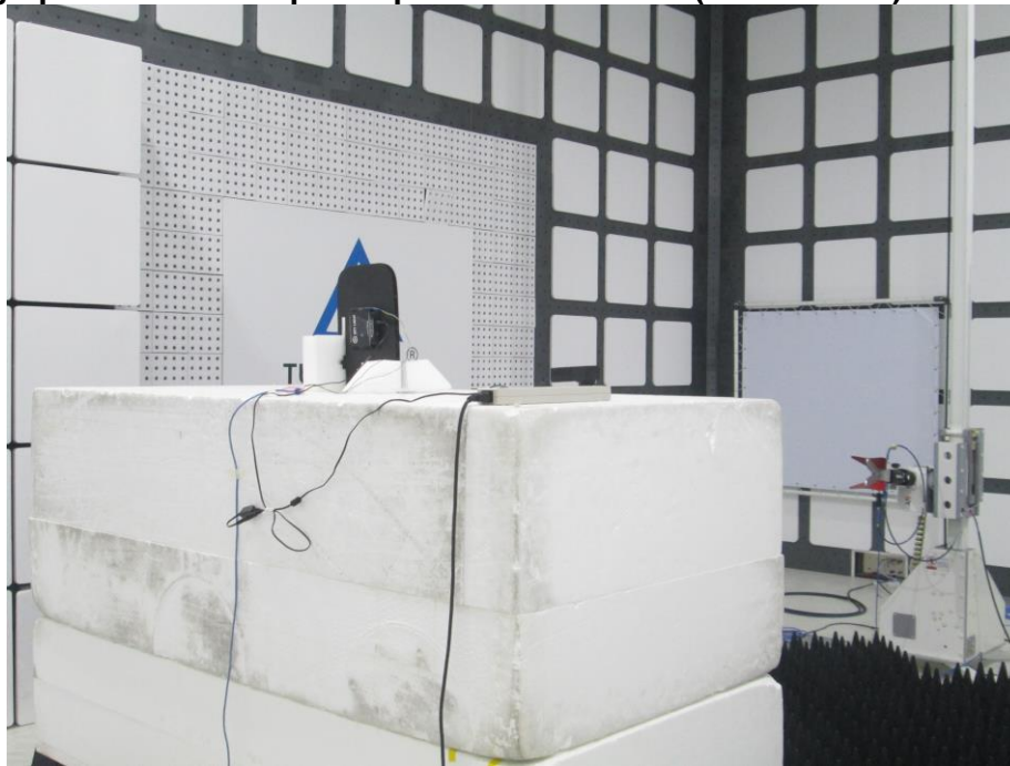
Photograph 14: Test Setup for Spurious Emissions (Back View 4)
