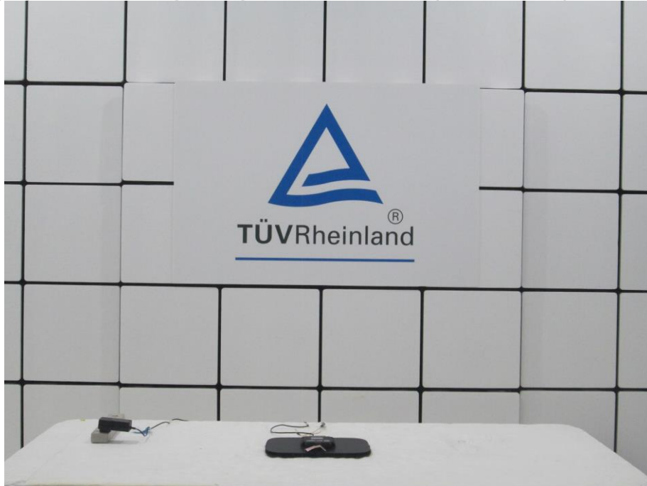
Photograph 1: Test Setup for Spurious Emissions (Front View 1)
