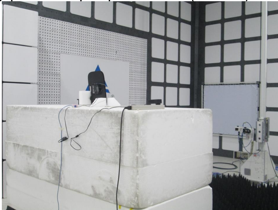
Photograph 14: Test Setup for Spurious Emissions (Back View 4)
