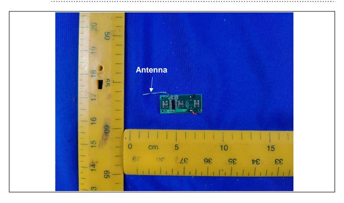
Details of: PCB view for remote controller
