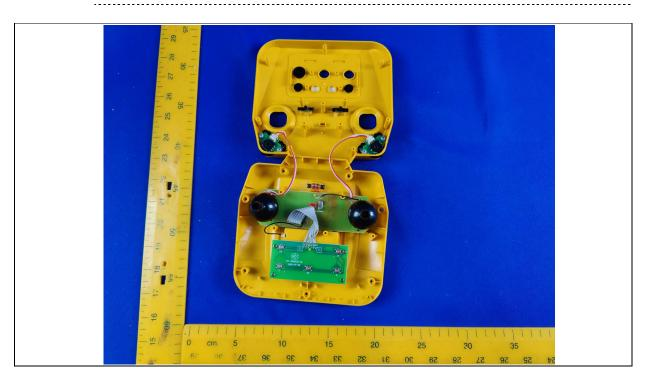
Details of: PCB view for remote controller
