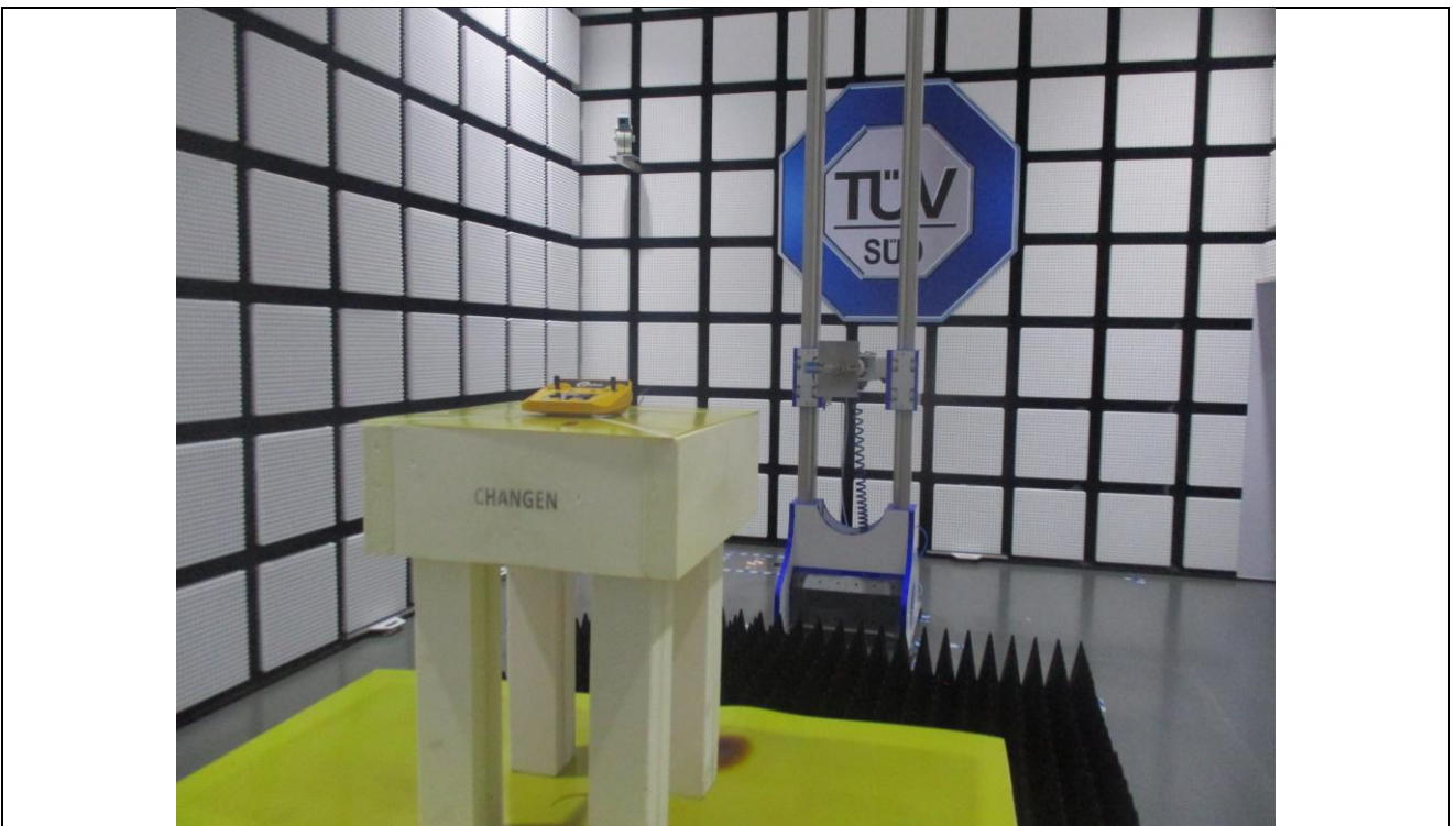
Radiated Emission test (1000MHz to 18000MHz)
