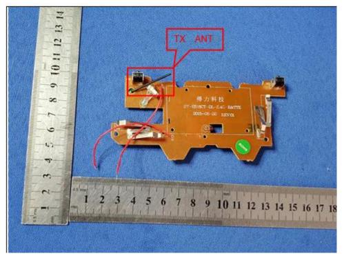
Length: 33mm Antenna Type: Wire Antenna Antenna Gain: 0dBi
