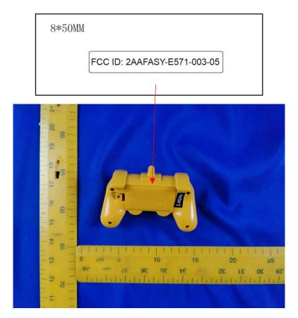
Stuck on the top surface of the remote controller
