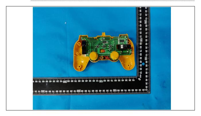
Details of: PCB view for remote controller
