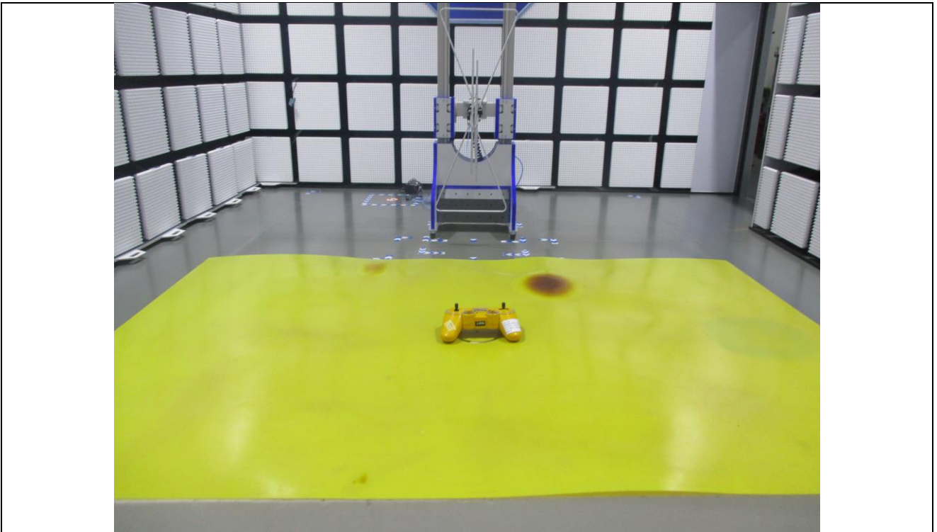
Radiated Emission test (30MHz to 1000MHz)
