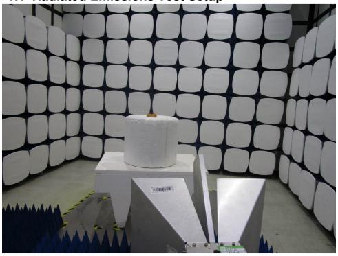
1.2 Radiated Emissions Test Setup
