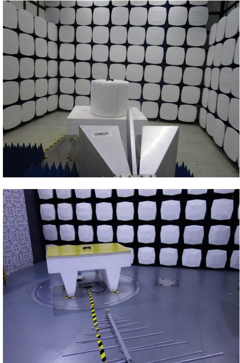
1.3 Radiated Emissions Test Setup
