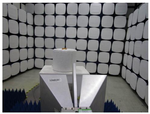
1.3 Radiated Emissions Test Setup
