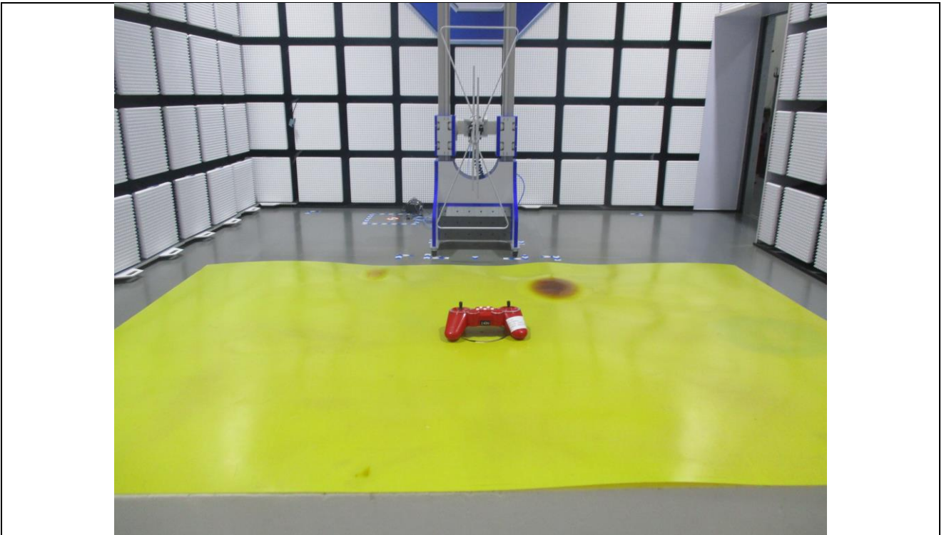
Radiated Emission test (30MHz to 1000MHz)
