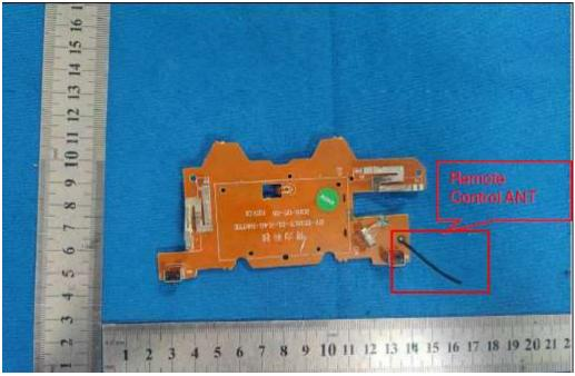
Length: 33mm Antenna Type: Wire Antenna Antenna Gain: 0dBi
