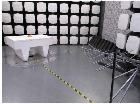
1.4 Radiated Emissions Test Setup (Above 1GHz)
