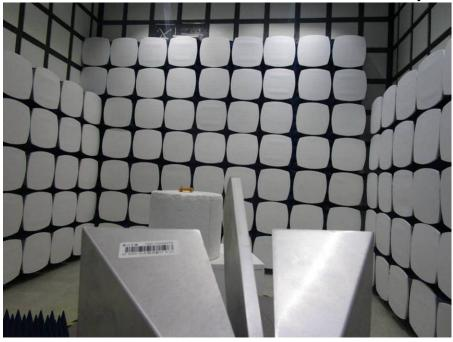
1.3 Radiated Emissions Test Setup (30MHz~1GHz)
