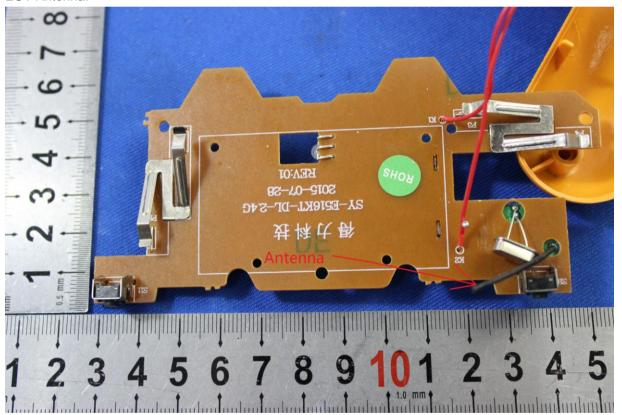
The antenna is integrated on the main PCB and no consideration of replacement. The best case gain of the antenna is 0 dBi.
