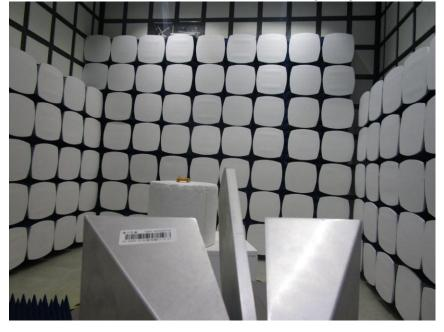
1.3 Radiated Emissions Test Setup(30MHz~1GHz)
