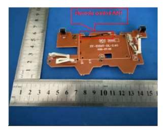
Length: 43mm Antenna Type: Wire Antenna Antenna Gain: 0dBi
