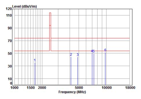
Condition: 3m VERTICAL Job No.: 05266CR Test mode: 2440 TX RSE
