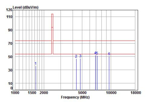
Condition: 3m VERTICAL Job No.: 05266CR Test mode: 2402 TX RSE
