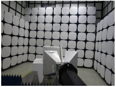
1.3 Radiated Emissions Test Setup (30MHz~1GHz)
