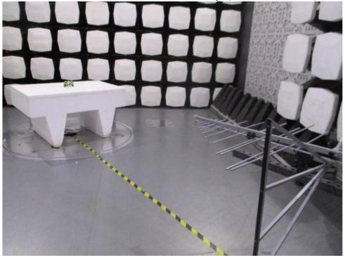
1.4 Radiated Emissions Test Setup (Above 1GHz)
