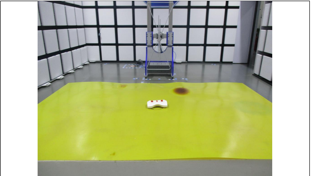
Radiated Emission test (30MHz to 1000MHz)
