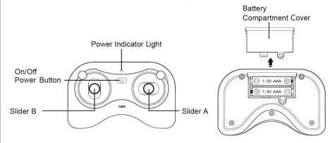
Install 2 pcs of 1.5V AAA non rechargeable batteries in the correct polarity (remote control batteries are not included).
