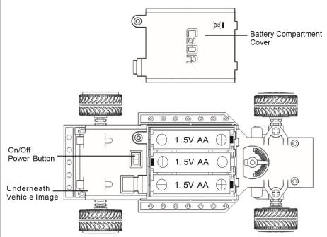
Install 3 pcs of 1.5V AA non rechargeable batteries in the correct polarity (vehicle batteries are not included).
