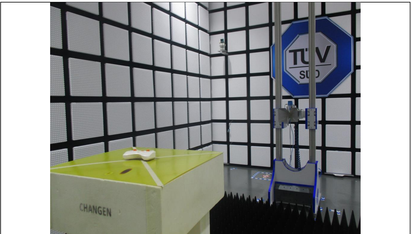
Radiated Emission test (1000MHz to 18000MHz)
