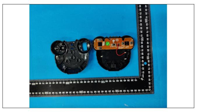
Details of: PCB view for Remote controller
