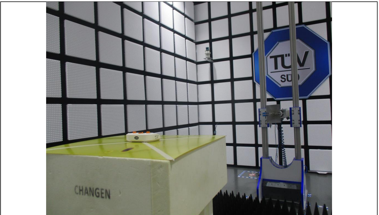
Radiated Emission test (1000MHz to 18000MHz)
