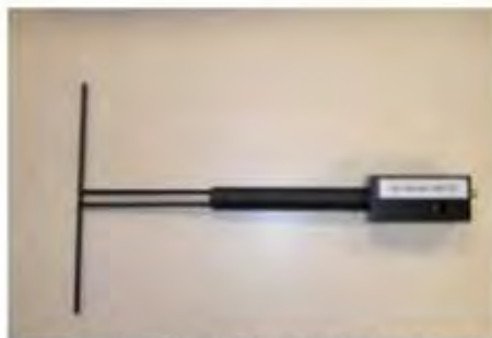
Figure 1 – Satimo COMOSAR Validation Dipole
