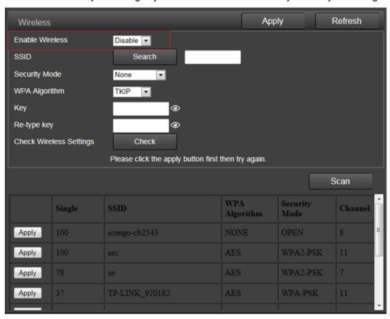
**Note:** The Dericam camera use the wired Ethernet cable by default, it will work on the wireless status automatically if you disconnect the Ethernet cable. But the wireless will not work if you still connect the Ethernet cable in your camera.
