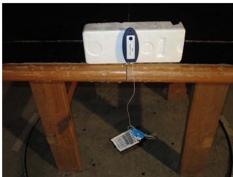
Photograph 8.1.6 Setup for final radiated emission measurements, U-Sensor close view
