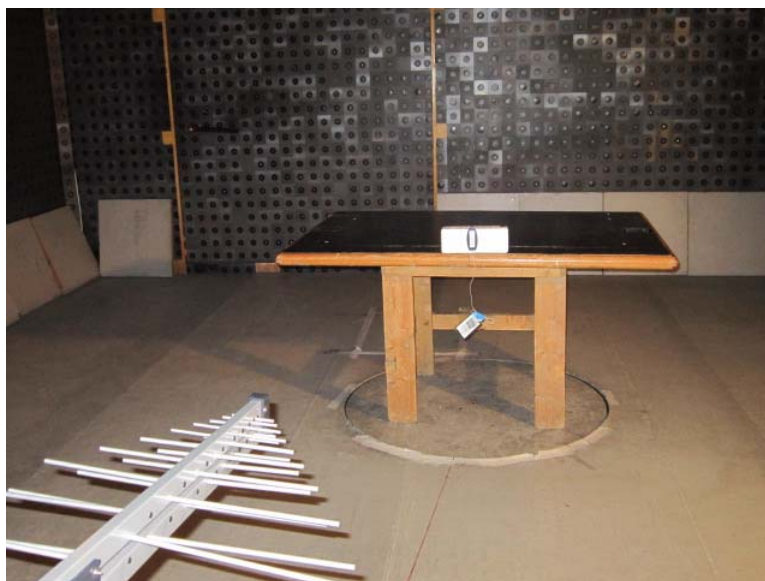
Photograph 8.1.4 Setup for radiated emission measurements of U-Sensor
