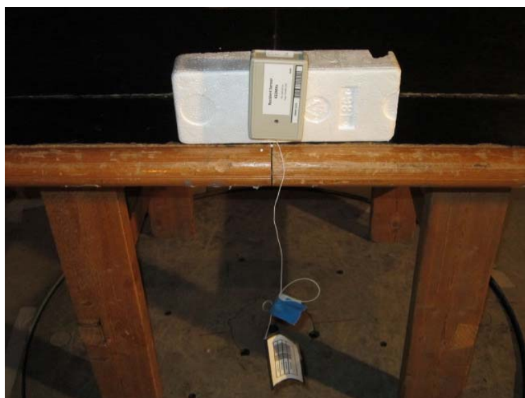
Photograph 8.1.3 Setup for final radiated emission measurements, R-Sensor close view
