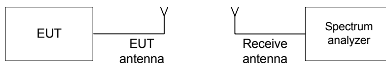
Figure 7.3.1 Occupied bandwidth test setup
