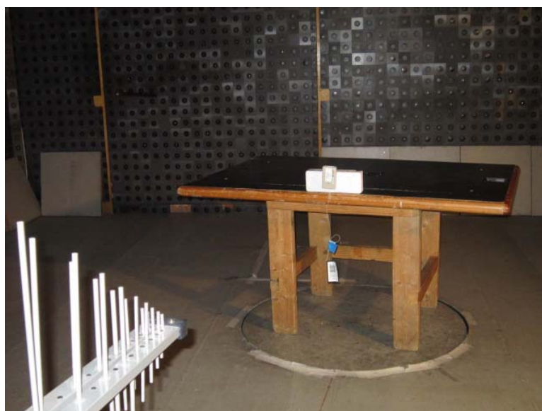
Photograph 8.1.2 Setup for radiated emission measurements of R-Sensor
