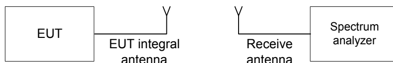
Figure 7.1.1 Setup for transmitter shut down test
