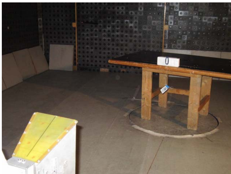
Photograph 8.1.5 Setup for radiated emission measurements of U-Sensor
