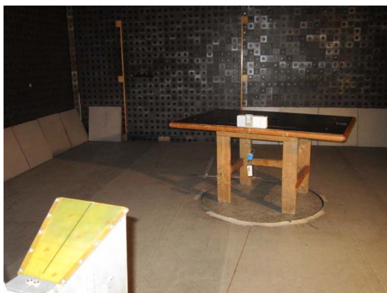
Photograph 8.1.2 Setup for radiated emission measurements of R-Sensor
